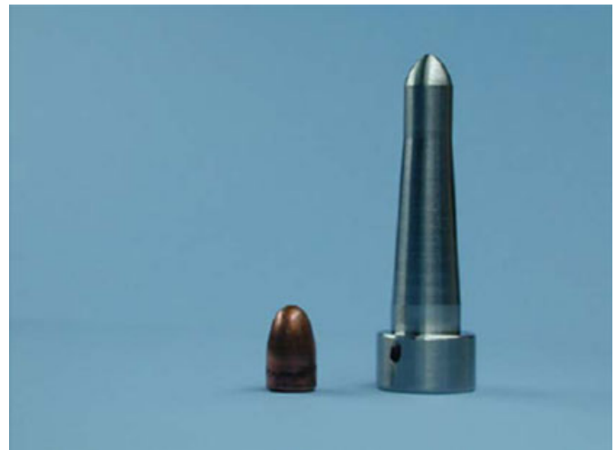
FIG. 5—Dropping weight impact head shown with 9-mm bullet.
